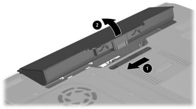
Removing the Battery Pack
